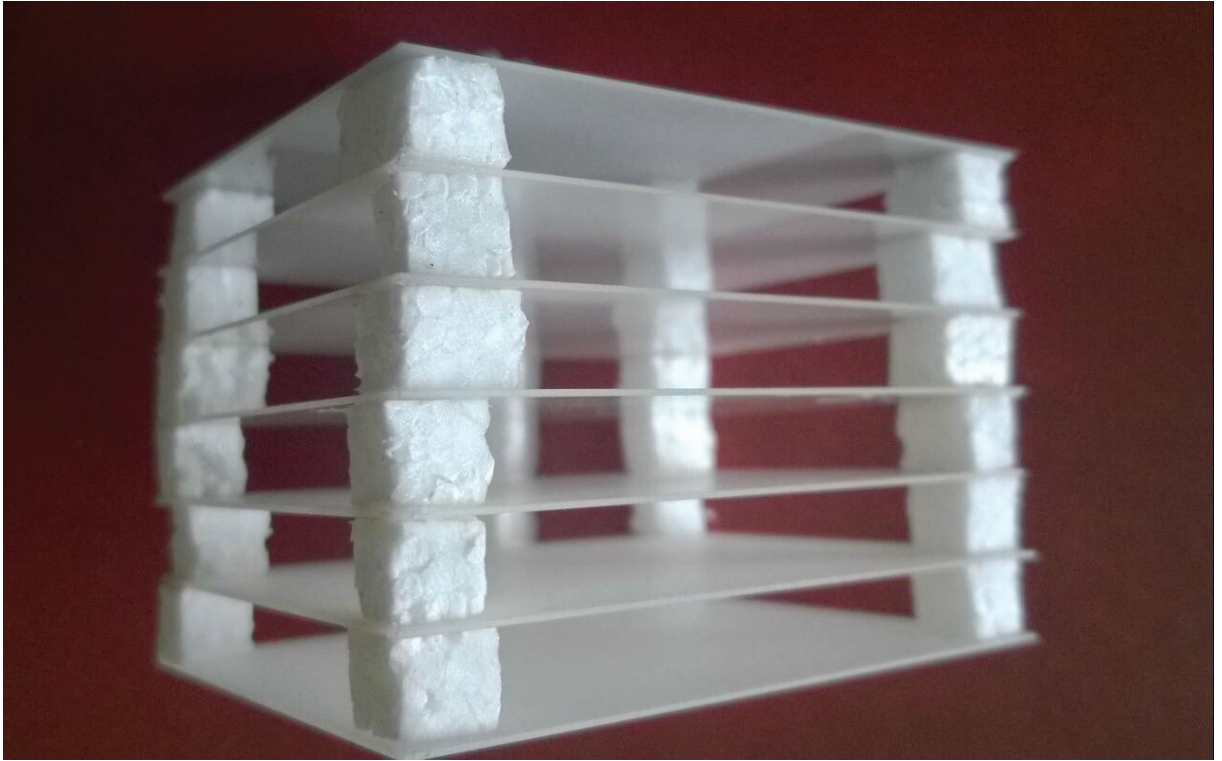
Figure 2: One dimensional photonic crystal. Photograph of the 1d PC used in the experiment. It is formed from 7 alumina ceramic plates with \varepsilon = 10 , thickness b = 0.5 mm, sizes 60 \times 96 \text{ mm}^2 and a = 10 mm distance from each other.
